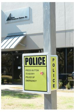
The large POLICE emergency weatherproof enclosure is wireless and battery powered; ideal for parking lots, garages and remote areas. This includes an enclosure mounting back plate, pole mounting bracket with fasteners, wall mount clips, poly carbonate enclosure, and weatherproof red duress button. When activated, a wireless alert is sent to the LynxGuide server via the LynxNet WLS.
