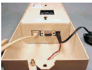
Bottom view of the unit showing the Network, RS-232 and Power connectors
